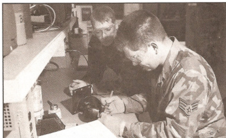
Senior Airman Charles Chambers and Staff Sgt. Richard Ebhardt solder a switch to a weapons controller.
